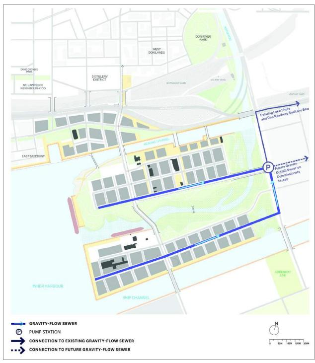
FIGURE 6-12 LDLMP EA STORMWATER DRAINAGE
