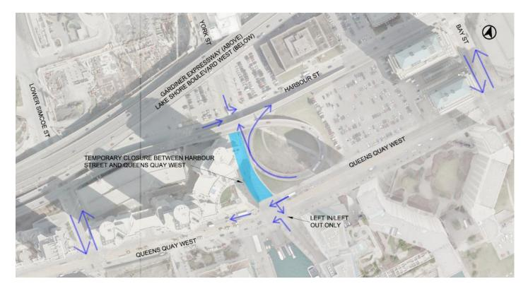
A temporary closure of York Street between Harbour Street and Queens Quay will be required from September 15 to October 3. This temporary street closure is required to connect the newly installed stormwater infrastructure on Queens Quay to the existing infrastructure on York Street.
