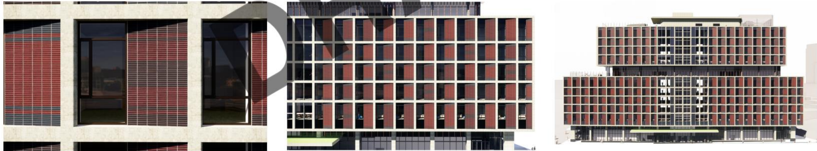
PRECAST BRICKSLIP PATTERN STUDY
