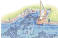
Sheltered Embayment: Inner Harbour Quay Restoration - Inner harbour quay treatments using structural habitat such as anchored logs, floating docks, and rock gravel shoals and reefs
