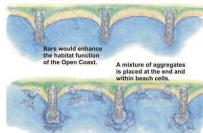
Open Coast - Surcharged Open Coast Groyne The additional substrate provides shoreline stability, and structural habitat associated with offshore shoals and bars would enhance the habitat function of the Open Coast.
