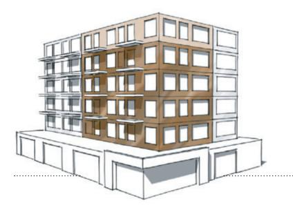
Simple, compact forms for buildings help to minimize thermal bridging through the building envelope.
