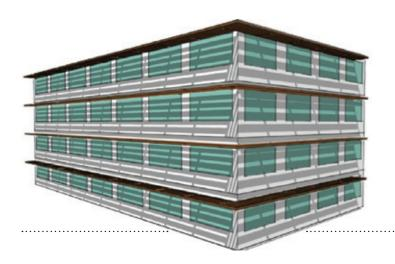
Shading devices installed over windows on south and west facades help to minimize solar gains in the summer months
