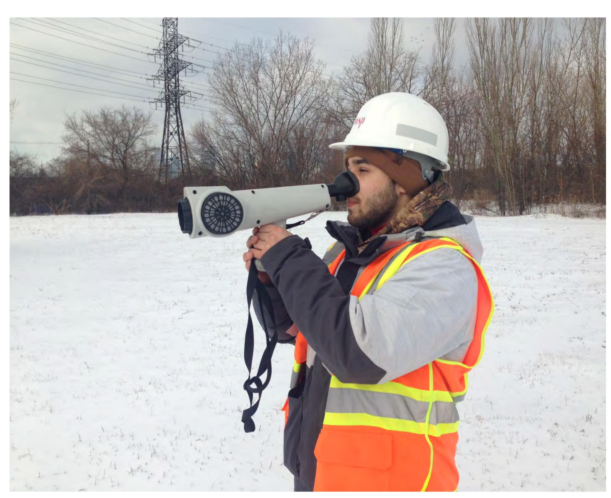
We use a nasal ranger or olfactometer to measure existing odour in and around the construction site.
