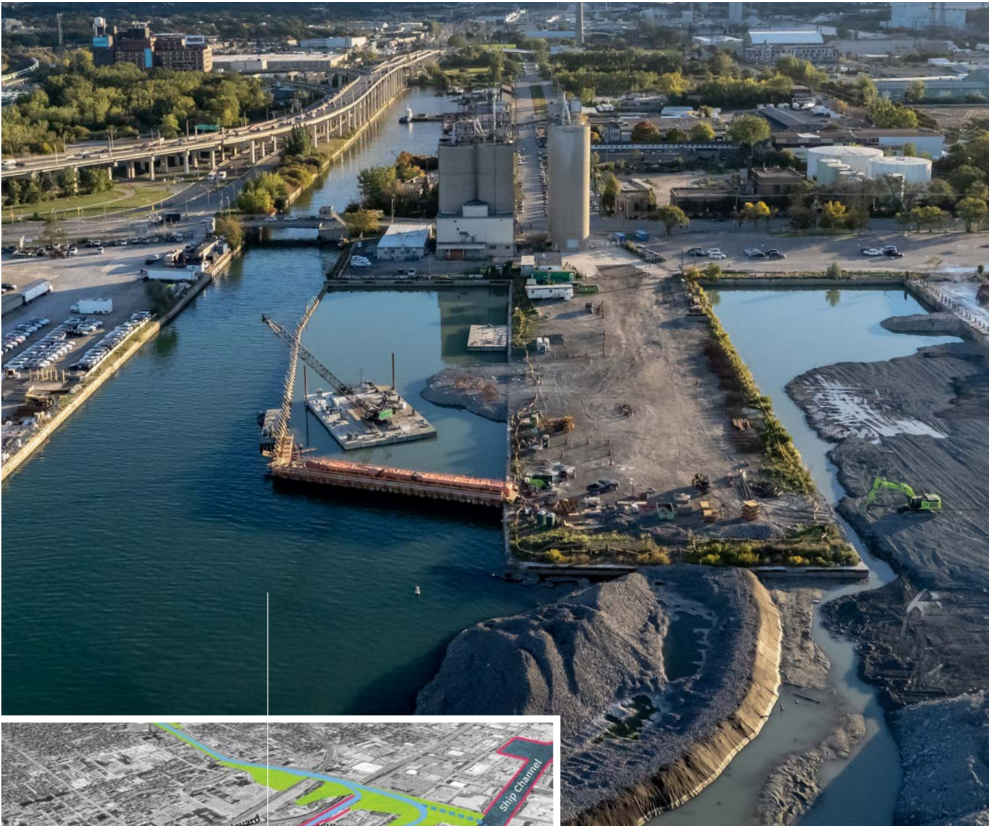
Larger image: lakefilling work associated with the Port Lands Flood Protection Project. Smaller image: the eventual course of the river when work is complete.
