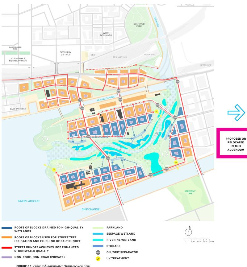
FIGURE 8.1: Proposed Stormwater Drainage Revisions
