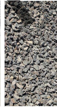
Rough Natural Stone Aggregate 2-4cm Dia. and 10-20cm Dia.
