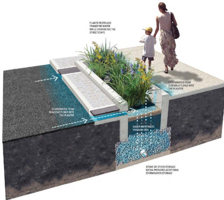
Example of a Stormwater Planter. Source: City of Philadelphia, Green Streets Design Manual
