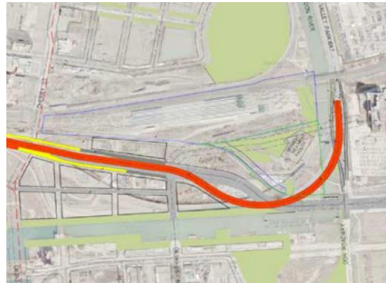
Hybrid ramp design with 70 km/hr design speed.
