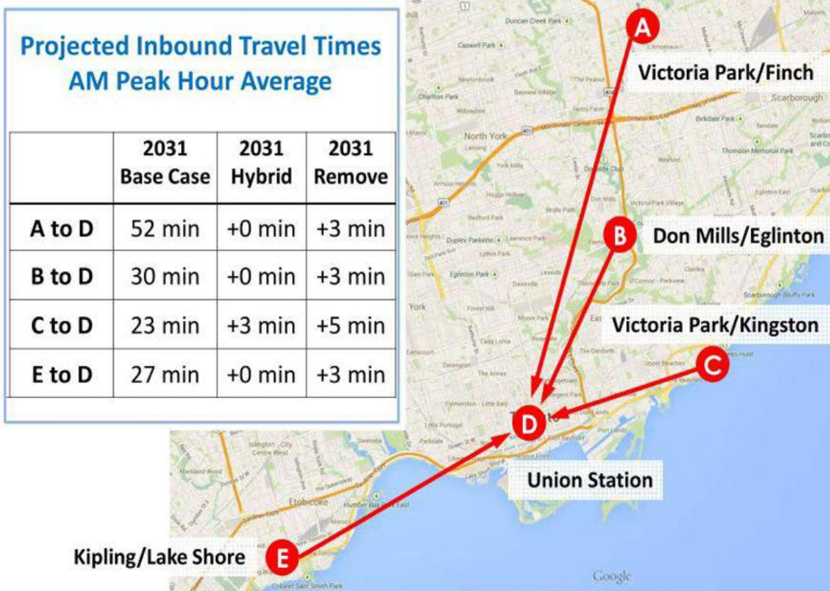
Figure 4.11: Auto Travel Times for Select OD Pairs for Hybrid and Optimized Remove
