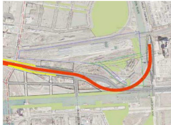
Hybrid ramp design with 70 km/hr design speed.
