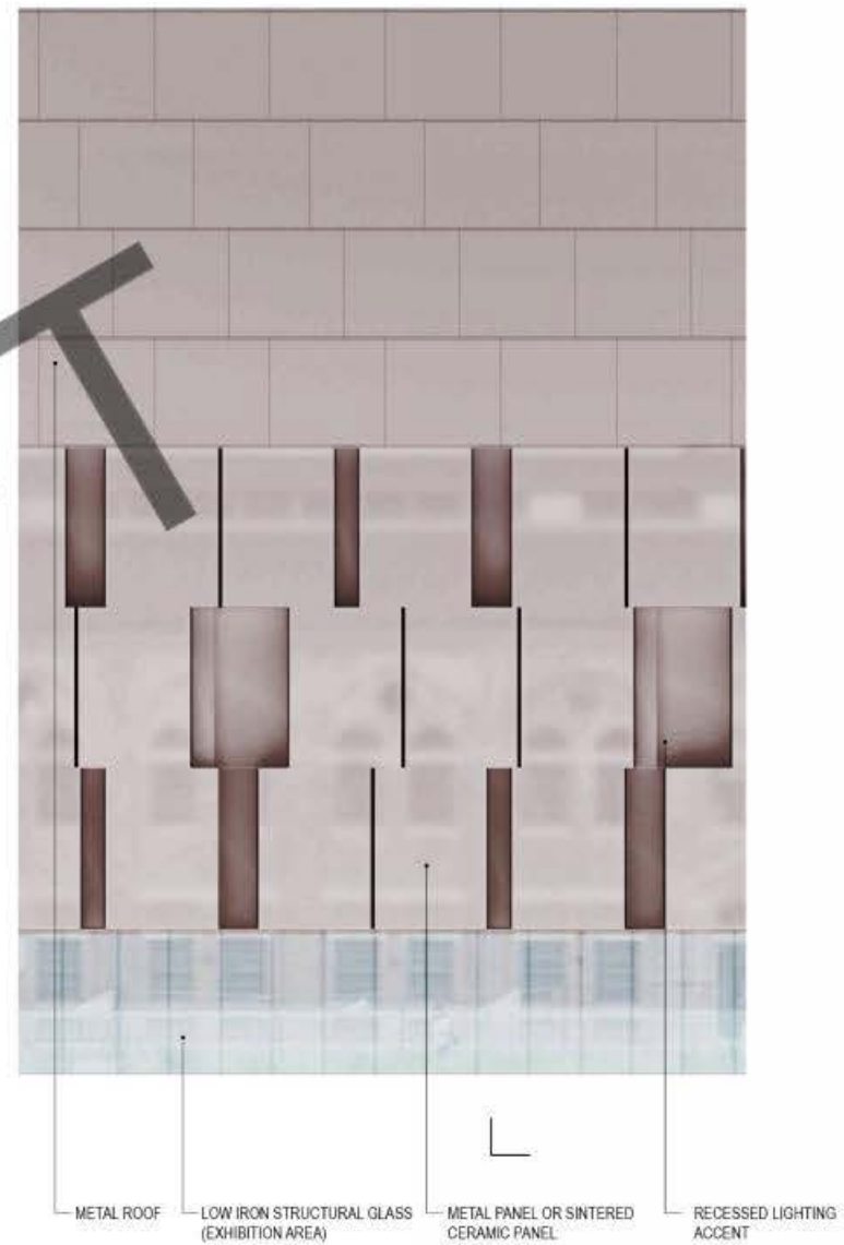
PARTIAL BUILDING SECTION
