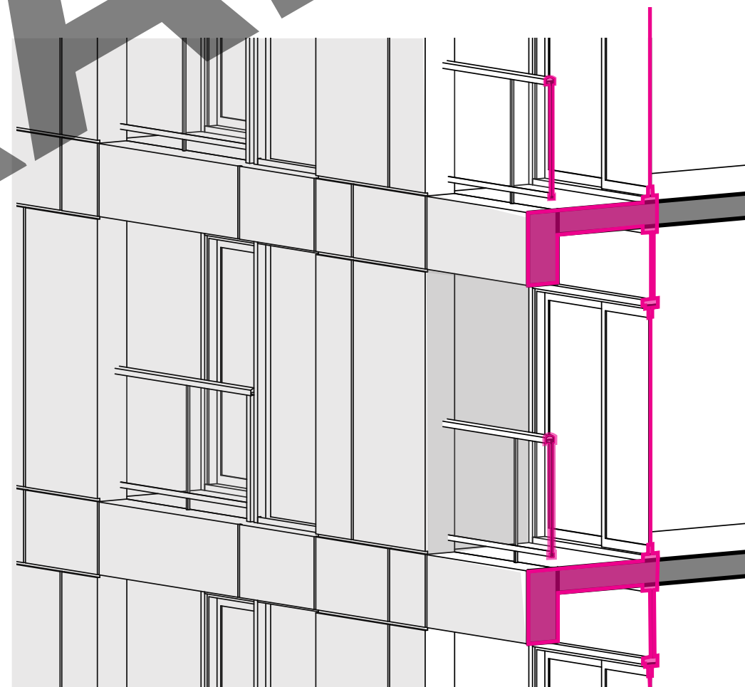
THERMAL BRIDGING (INSET BALCONIES)
