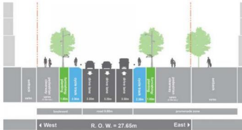
Figure 2.3 Yonge Street: South of Harbour Street 3-Lane + Uni-directional Cycle Tracks (27.65m R.O.W.) Note: Raised cycle tracks with fully mountable curb. From the Lower Yonge Municipal Class EA process.
