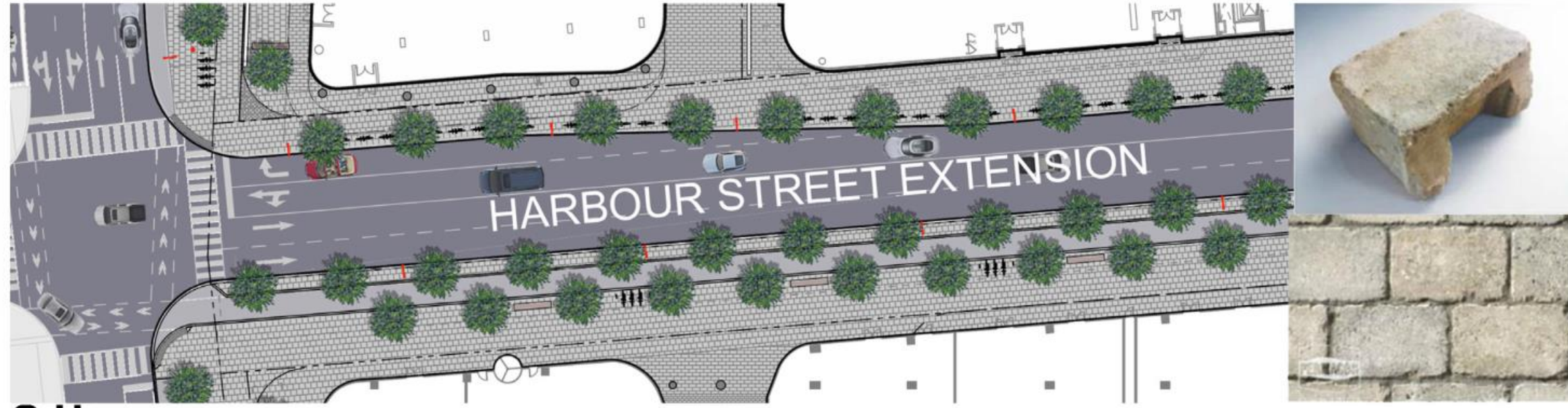
2. Harbour Street Paving (140x220x100mm Silex Grey Interlocking concrete pavers)
