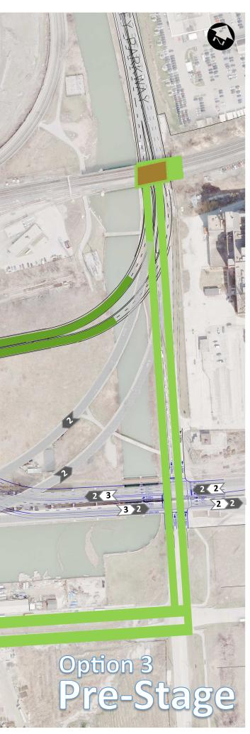
Demolish S/W DVP ramp, FGE WBL (including Logan Ramp), Don River bridge WB, and existing LSB WBL
