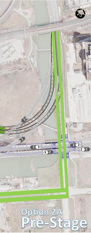
Demolish S/W DVP ramp, FGE WBL (including Logan Ramp), Don River bridge WB, and existing LSB WBL Construct new S/W DVP ramp, FGE WBL ramp, Don
