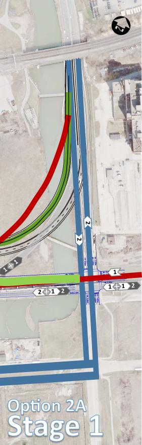
Demolish E/N DVP ramp, FGE EBL (including Logan Ramp), Don River bridge EB, and existing LSB EBL
