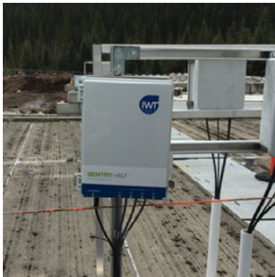
SENTRY, a bio-electrode microbial activity and water quality monitoring platform. Source: https://techhub.wwf.ca/innovator/real-time-bio-electrode-monitoring-of-water-environments/
