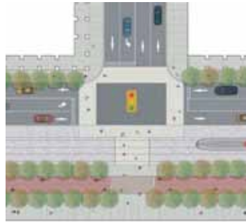
Two-Phase Pedestrian Activated Crossing
