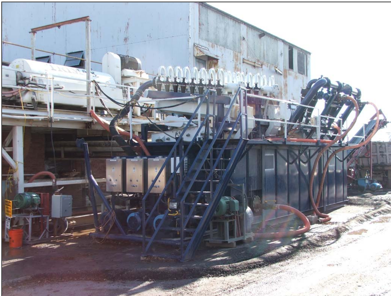
Soil washing Photo source: Biogenesis
