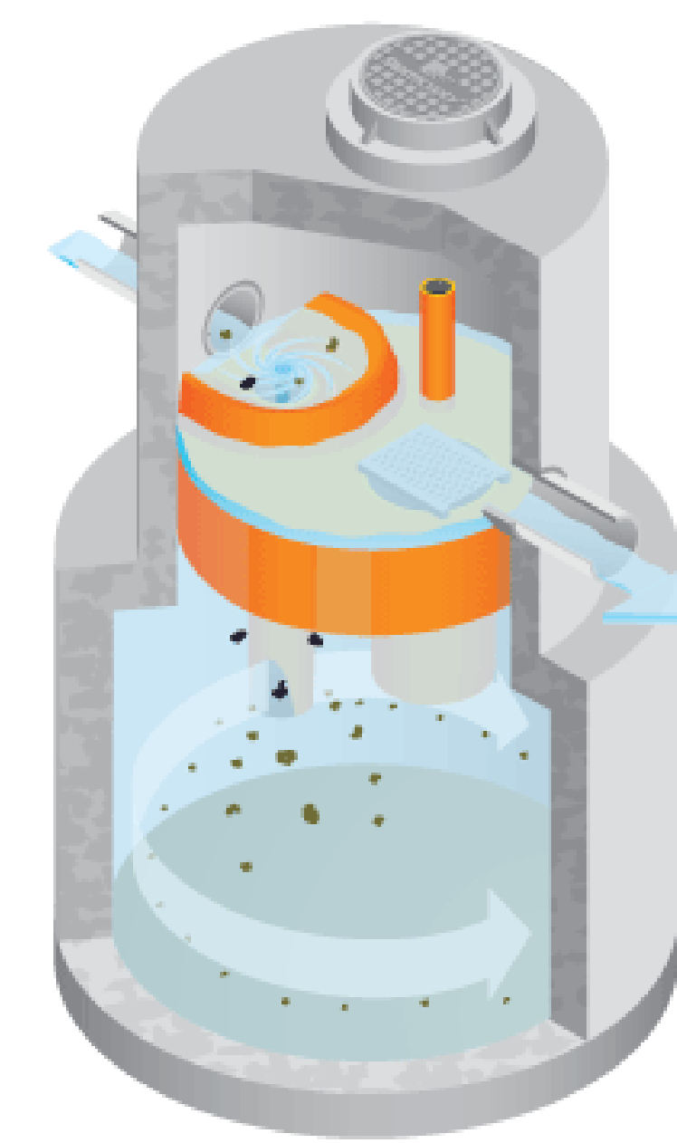
A typical water quality manhole (oil-grit separator)
