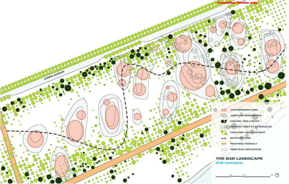
conceptual design response to isolated levels of soil contamination
