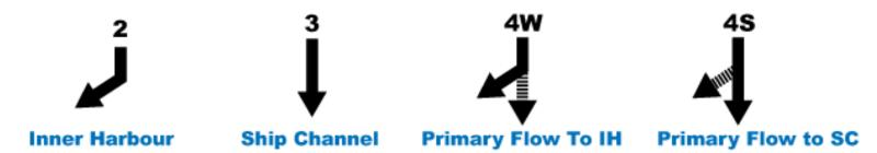
The ToR defines Alternative 4 (W and S) as having one primary channel (assumed 300 m wide) and one regional overflow channel (200 - 300 m wide). Alternatives 3 and 4S envisioned the Don Greenway as a river mouth, providing both greenway and naturalized river mouth functions. Alternative 4W aligns the greenway with a proposed overflow spillway function.
