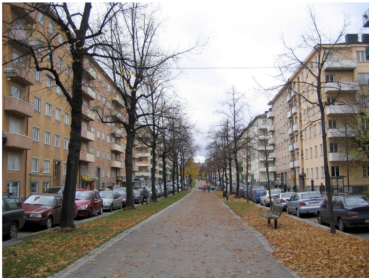
Figure 2:7 An example of a separate Path for Pedestrians and Bicyclists centrally located in a Street Space. Erik Dahlbergsgatan in Stockholm.
