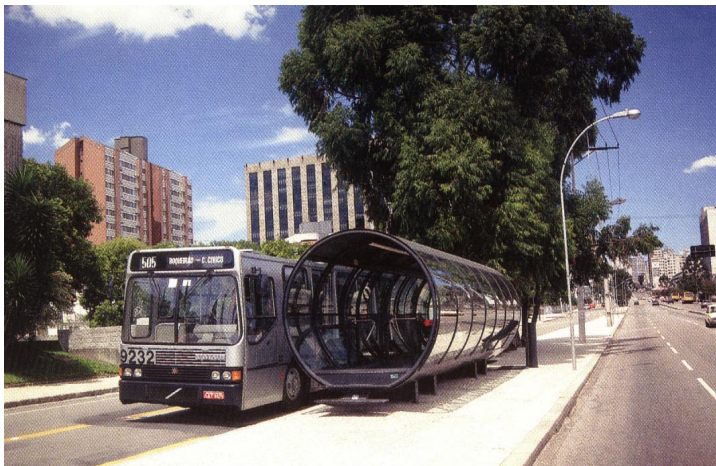
Figure 2:4 The Curitiba Example in Brazil. A Bus-Stop along a separate Lane for Express Buses.
