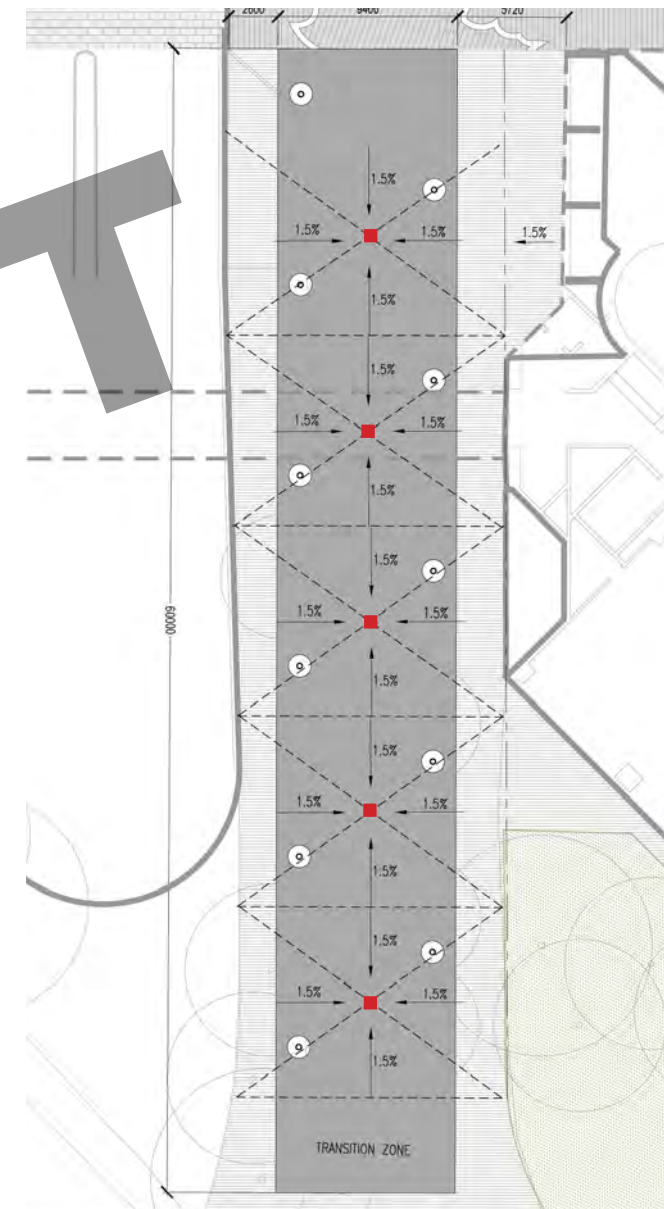
C the use of inlet's or CB's in the center of the promenade (reference Sugar Beach)
