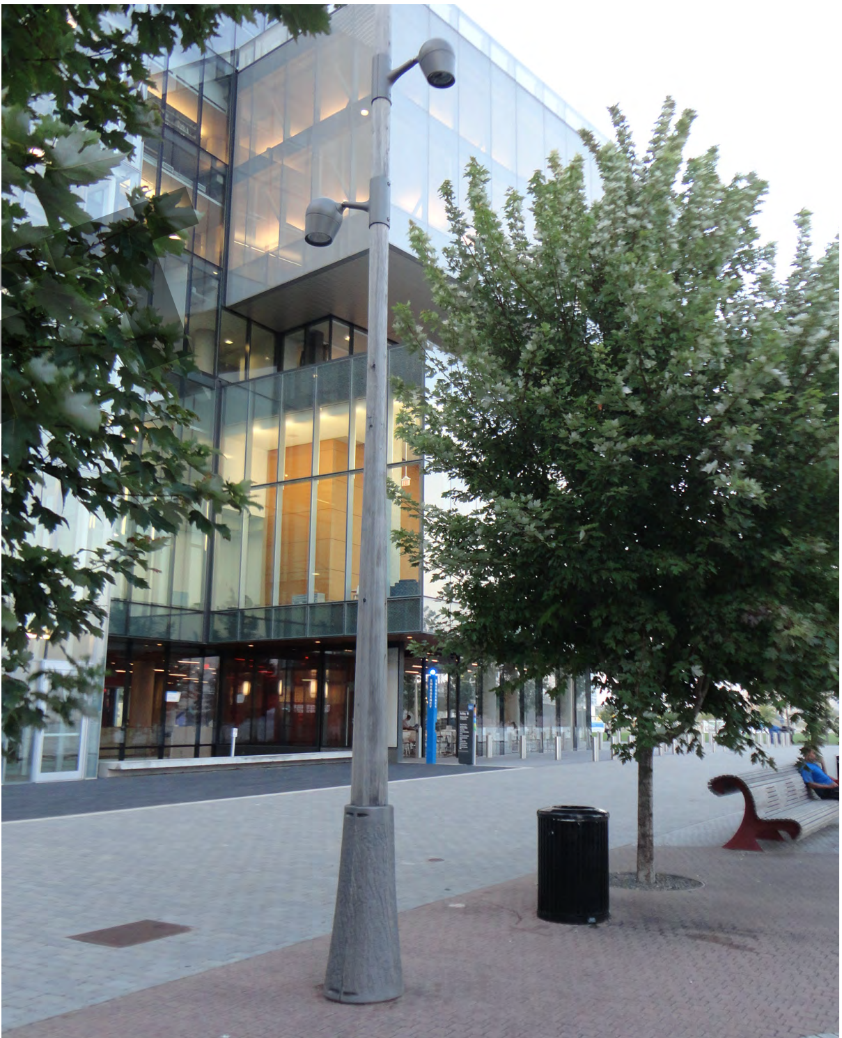
Waterfront Toronto signature light pole 6m high with Olivio light feature and shroud
