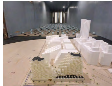
Study model inside the GWE wind tunnel.
