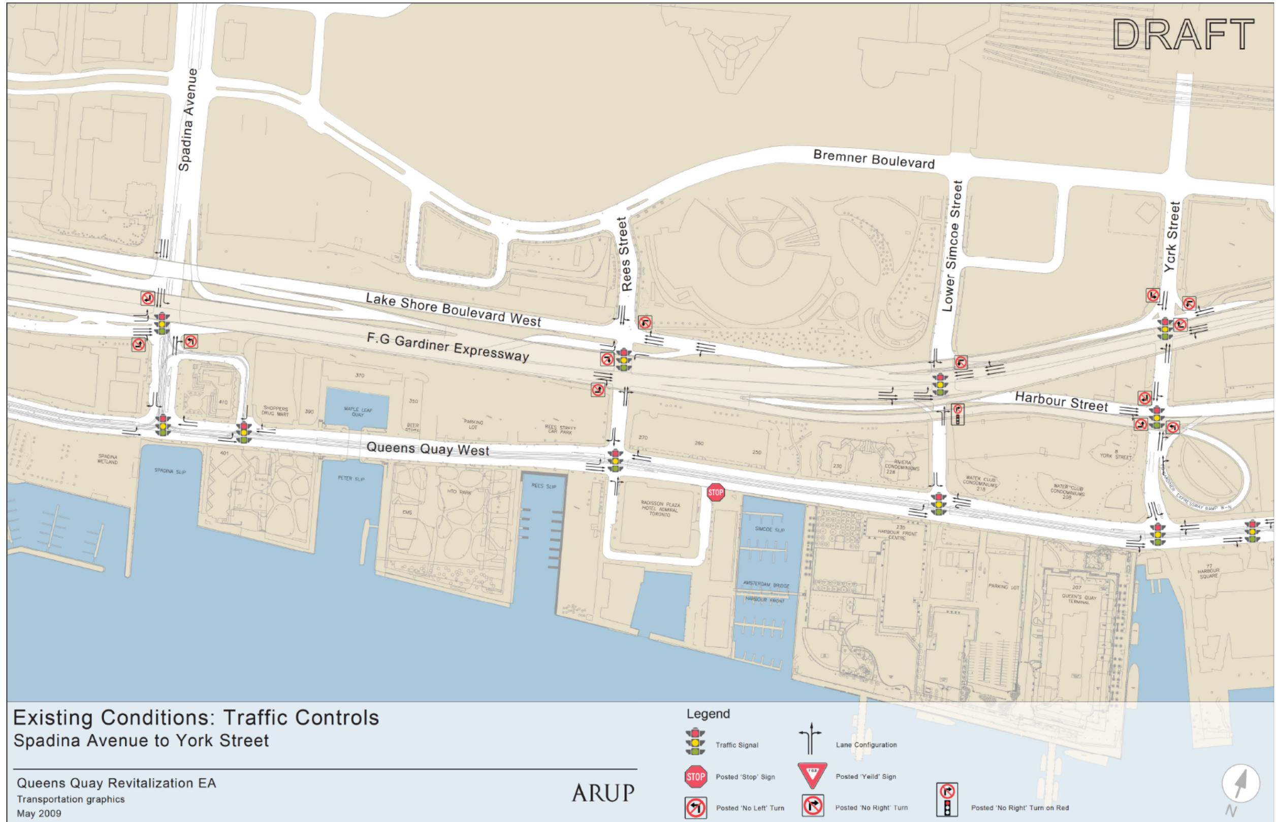
Figure 5-13: Existing Intersection Traffic Control East
