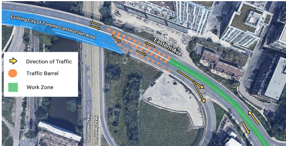
Above: Aerial shot of Eastern Avenue near the Don Valley Parkway, showing work zones, traffic flow, and temporary traffic control using barrels.
