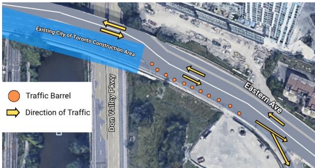
Above: Aerial shot of Eastern Avenue showing the use of traffic guides (orange markers) to section off mobilization
