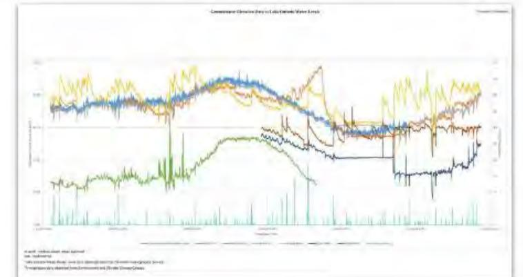
**Shallow Groundwater Monitoring** confirmed groundwater level fluctuates according to lake level → raised tree planters on QQE for resiliency
