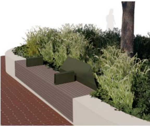
WOODEN BENCH : MODIFIED VERSION OF LANDSCAPE FORMS PARALLEL 42 BENCH EMBEDDED INTO CONCRETE PLANTER WALL (WITH OR WITHOUT METAL BACKREST AND ARMREST)
